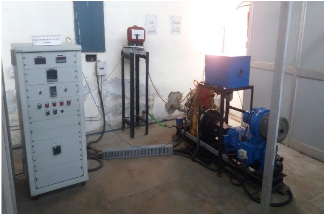
Figure 1. Test setup single cylinder VCR engine.
