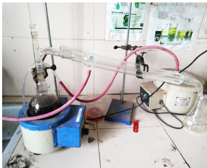
Figure 4. Distillation of black liquor.
