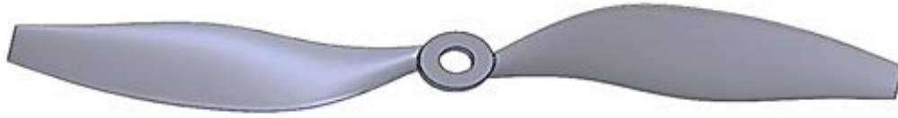
Figure 1. 3D CAD model of 7" NACA 4412 air foil propeller.
