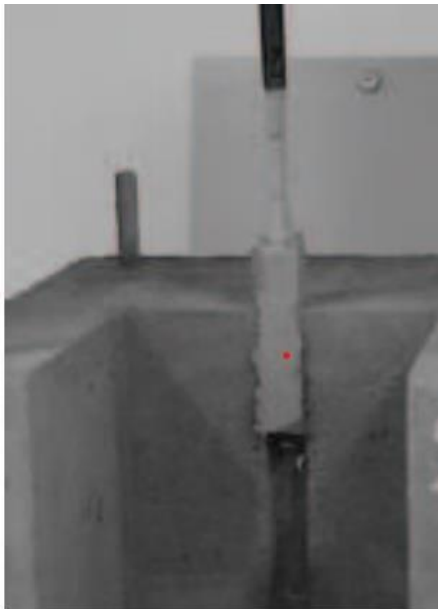
Figure 2. Failure at epoxy concrete interface.
