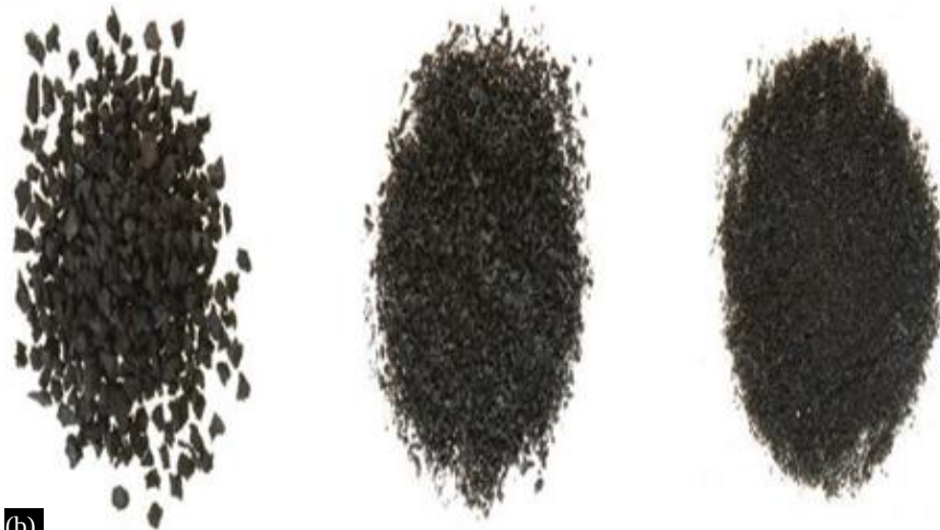
Figure 2. (a) Process of making fine and coarse rubber aggregate (10) (b) End product of tire rubber (11).
