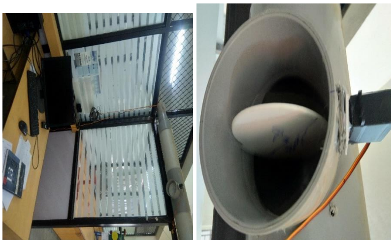
Figure 11. Installation of the Servo Motor with the Flipper in the Cabin.
