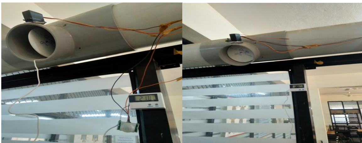
Figure 12. Digital thermostats observing the temperature of the cabin.
