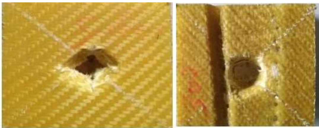
Figure 6. (a) Conventional Kevlar Sandwich panel at 25J, (b) Corrugated Kevlar sandwich panel at 25J and (c) Load Vs time graph at 25 J of conventional and corrugated Kevlar sandwich panel.
