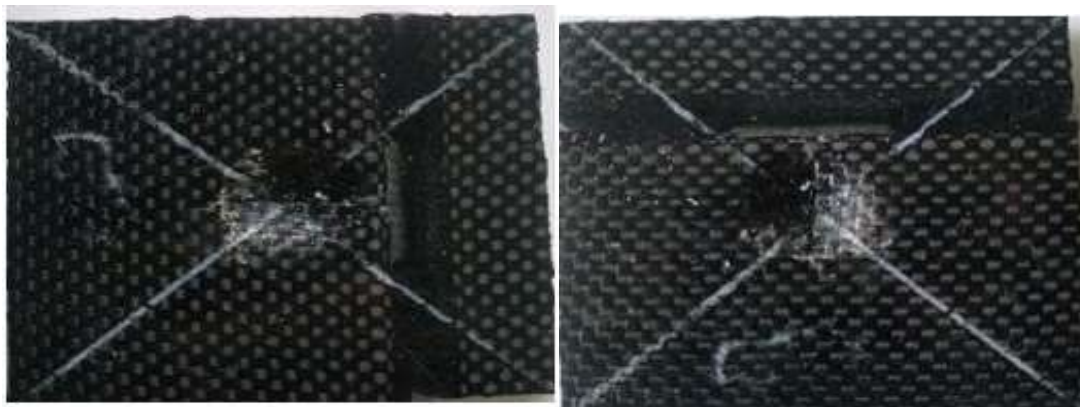
Figure 12. (a) Glass corrugated sandwich panel at 30 J, (b) Back view of the glass corrugated sandwich panel at 30 J and (c) Load Vs time graph of corrugated glass sandwich panel at 30 J.
