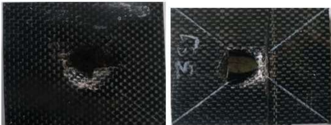
Figure 16. (a) Conventional carbon sandwich panel at 30 J, (b) Corrugated carbon sandwich panel at 30J and (c) Load Vs time graph of conventional and corrugated carbon sandwich panel at 30 J.
