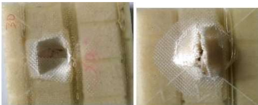
Figure 11. (a) Glass corrugated Sandwich panel at 25 J and (b) Load Vs time graph at 25 J of corrugated Glass sandwich panel.
