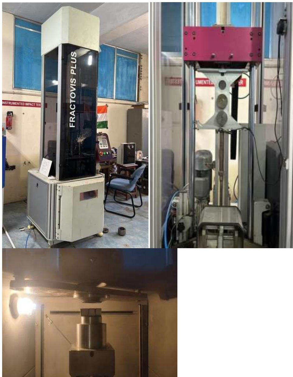
Figure 3. Impact test Facilities (a) Outer view of the Low velocity impact test facility, (b) Inner view of the Low velocity impact test facility and (c) Specimen on the steel hemispherical impactor.
