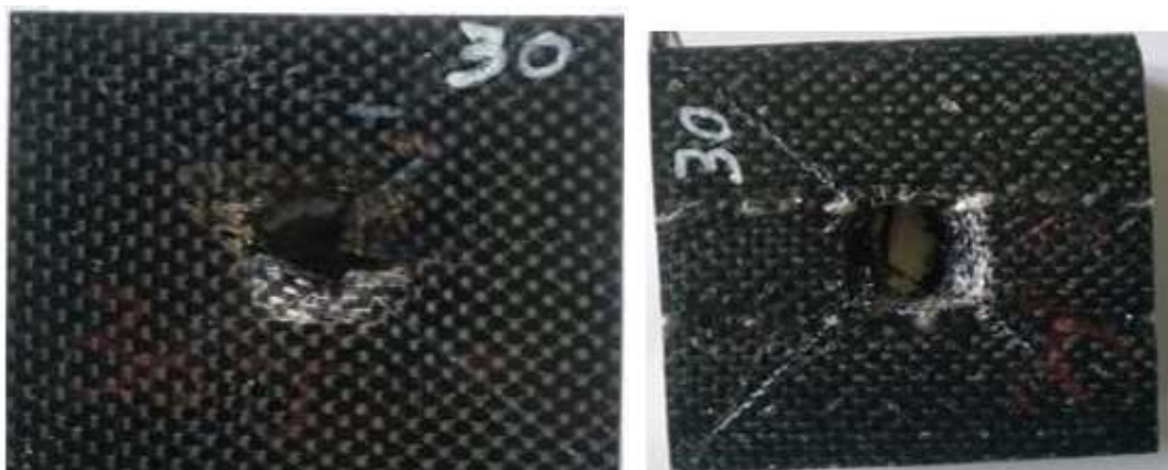
Figure 15. (a) Conventional carbon sandwich panel at 25J, (b) Corrugated carbon sandwich panel at 25J and (c) Load Vs time graph of conventional and corrugated carbon sandwich panel at 25 J.
