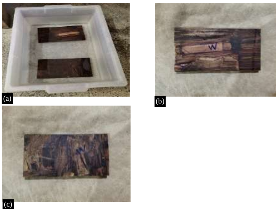
Figure 5. Board Preparation for Water Absorption Test (a) Water Absorption Test (b) Long Fiber Board (c) Short Fiber Board.
