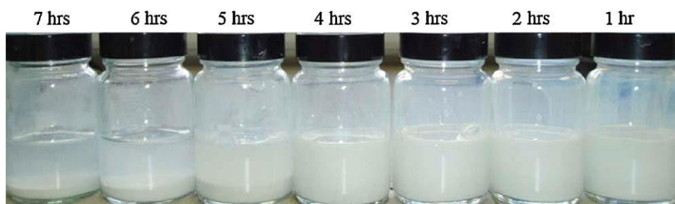
Figure 1. Samples of \text{Al}_2\text{O}_3 Nano fluids stability change with time [3].
