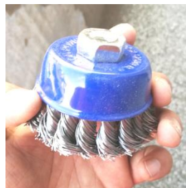
Fig. 6 Steel brush for sugarcane husk removal
