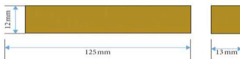
Figure 10. Geometry of the Flexural test specimen prepared as per ASTM.
