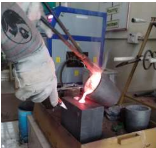
Figure 4. The composites were made using a stir casting setup.
