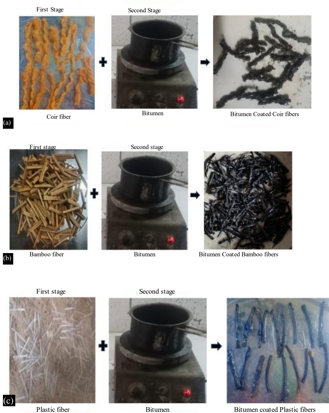
Figure 1. coated fibers (a) coir fibers, (b) Bamboo fibers and (c) Plastic fiber
