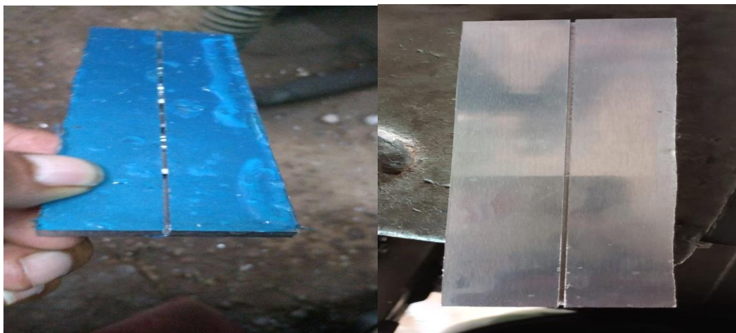
Figure 2. Base material after making groove
