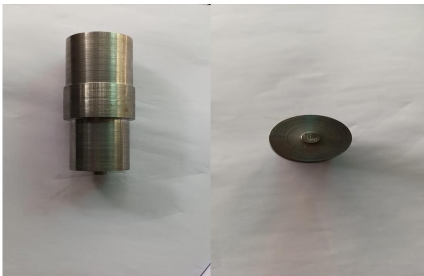
Figure 1. Single pin tool in different views
