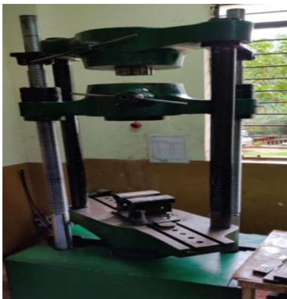
Figure 7. Tensile/shear load test before loading work piece
