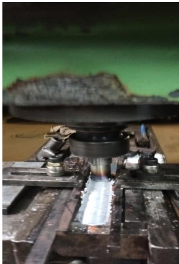
Figure 3. Machining using single pin tool
