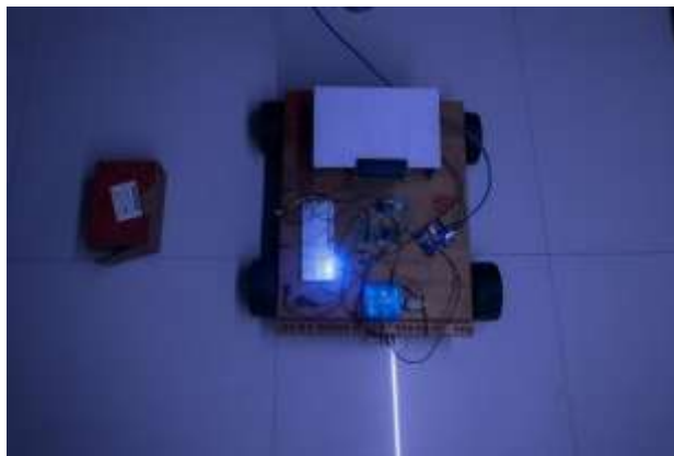
Fig.5. Rear sensor detection — Blue LED activated (obstacle within 50 cm)
