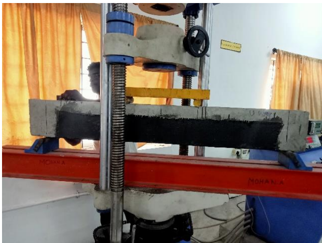
Figure 3. Hybrid U-wrap testing.
