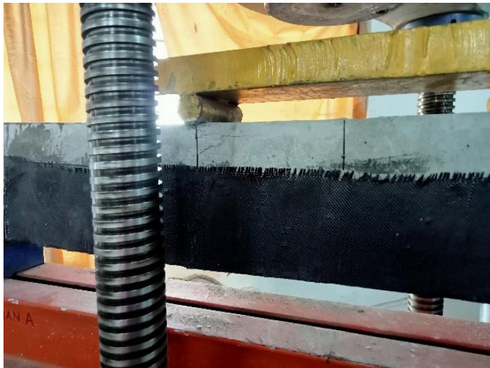
Figure 6. Hybrid crack patterns.
