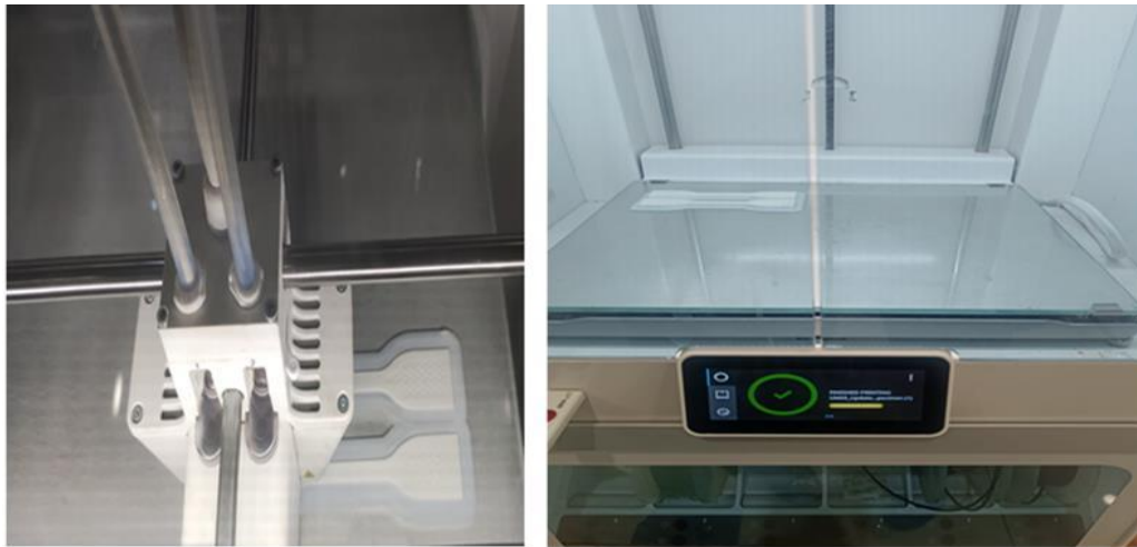
Figure 3. Printing of tensile test specimens on build platform at START position by FDM.
