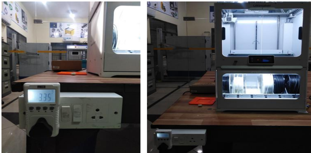
Figure 2. Measuring the readings for energy consumption & CO 2 emission of FDM during specimen printing with MECO power guard meter.
