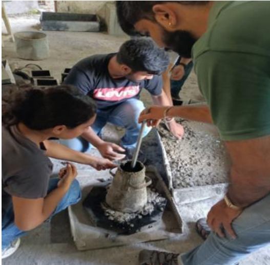
Figure 3. Filling of slump cone with fresh concrete.
