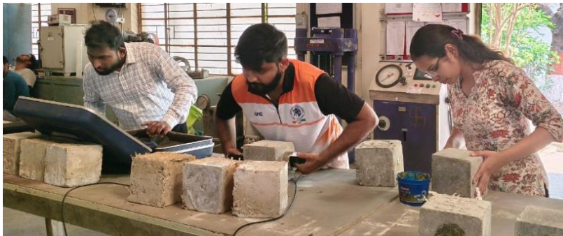
Figure 8. UPV (Ultrasonic Pulse Velocity) test on control and PET mix specimen durability (acid attack) test.
