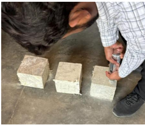
Figure 7. Rebound hammer test on control mix and PET mix specimen.
