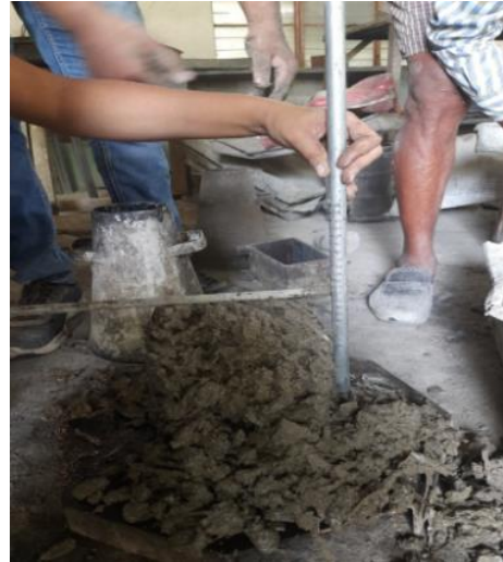
Figure 4. Measuring the slump value of fresh concrete and noticing its nature.
