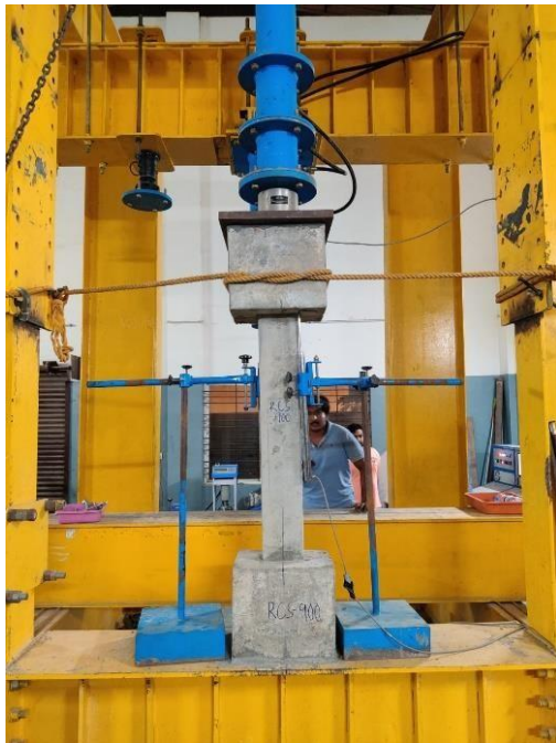
Figure 19. RCS900 specimen before testing CFRP WRAPPED SPECIMENS
