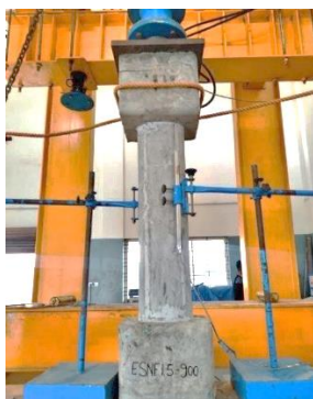
Figure 21. ESNF 1.5-900 before testing
