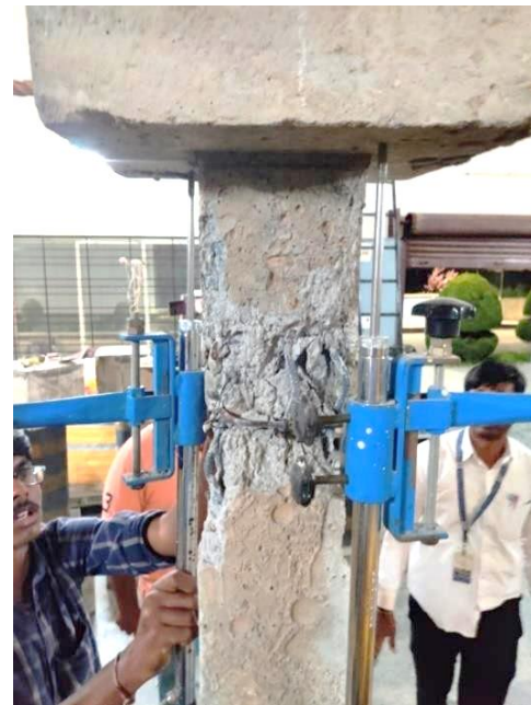
Figure 20. RCS900 specimen after testing
