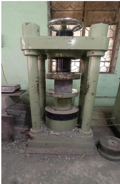
Figure 2. Testing of Cube in Compression.
