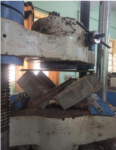
Figure 5. Failure Pattern of Prism in Flexure.
