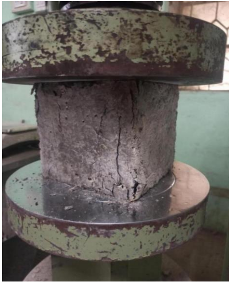
Figure 3. Failure Pattern of Cube in Compression.
