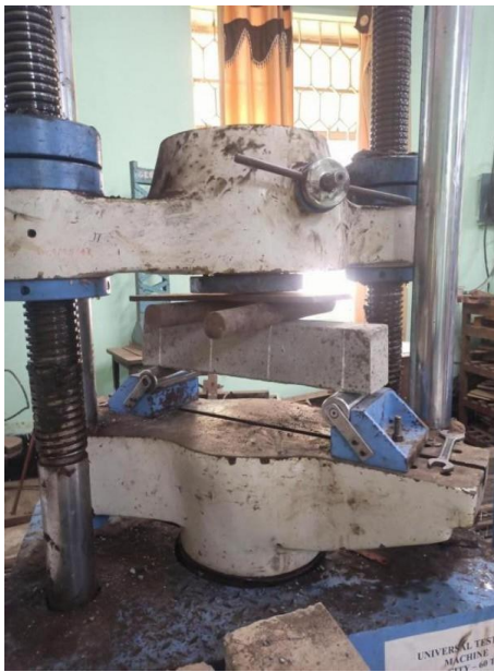
Figure 4. Test Setup for Flexure Test.
