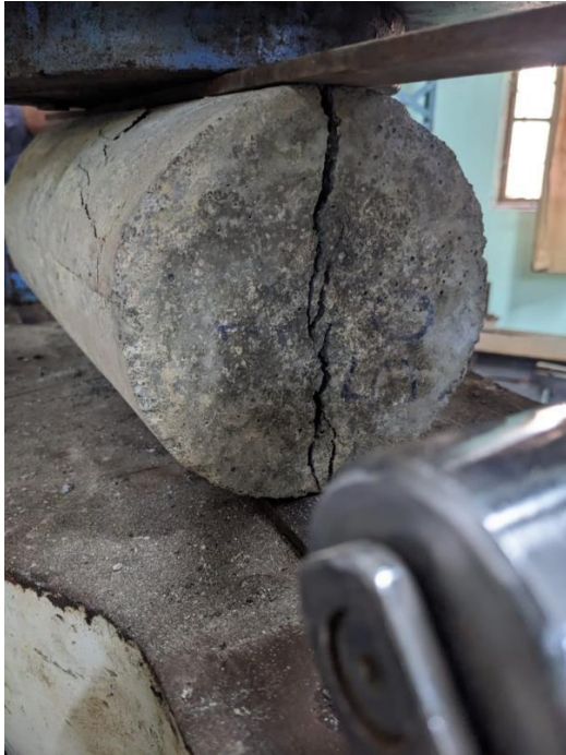
Figure 7. Failure pattern of Specimen in Split Tensile Test.
