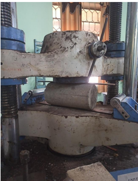
Figure 6. Test Setup for Split Tensile Test.
