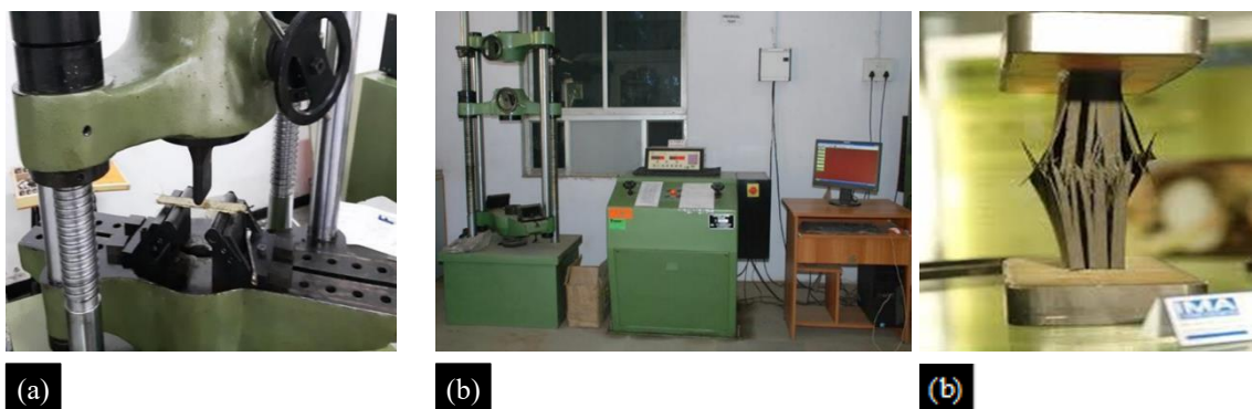
Figure 2. Experimental Setup and Failure Observation of Composite Samples (a) Flexural test machine, (b) Universal Testing Machine (UTM), (c) Delamination
