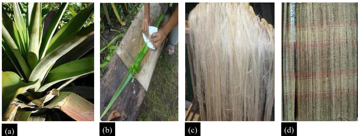
Figure 1. Preparation of Pine Apple Fiber (a) Harvesting Pineapple Leaves, (b) Fiber Extraction, (c) Washing and Cleaning, (d) Drying the Fibers
