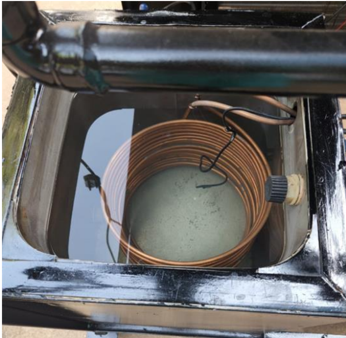
Figure 3. Developed evaporator inside refrigerated water tank.
