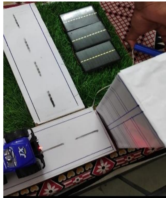
Figure 10. Output of solar wireless EV charging system (LED glows).
