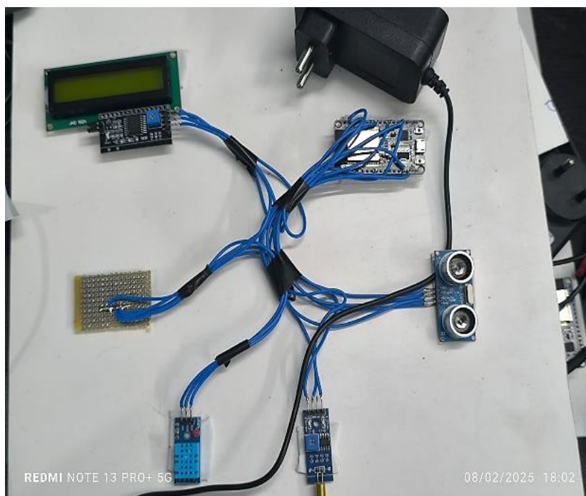
Figure 8. Final model of IoT based health monitoring system.
