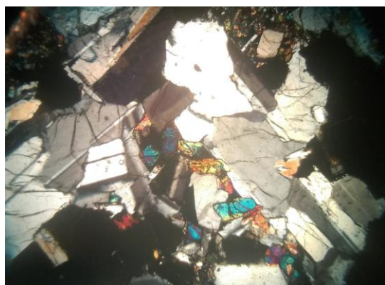
Figure 2. Sub-ophitic texture in basalt (augite partially enclosing plagioclase).
