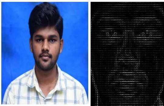
Figure 13. Result after performing histogram of oriented gradients (HOG) algorithm.
