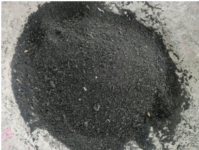
Figure 2. Fine aggregate as crumb rubber.
