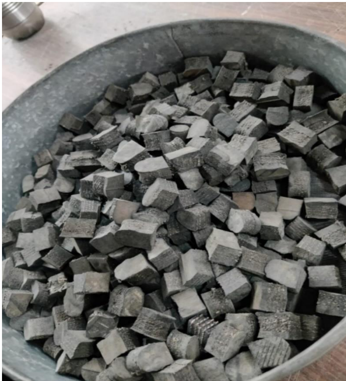
Figure 1. Crumb rubber as coarse aggregate.
