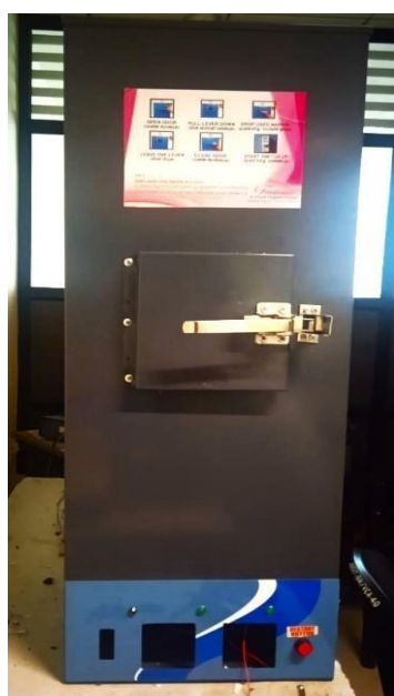
Figure 7. Final setup of proposed incinerator.
