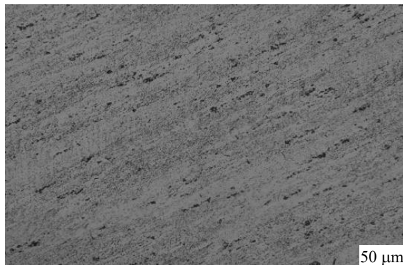
Figure 3. AA5083 has received, as measured by optical microstructure [19].
