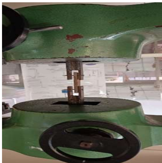
Figure 3. Sample subjected to tensile loading.
