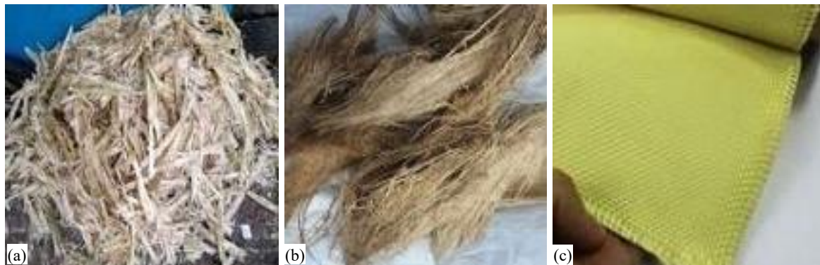
Figure 1. Pictorial view of (a) Sugarcane bagasse fiber, (b) Coconut fiber and (c) Kevlar fibre.
