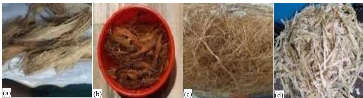
Figure 3. Coconut fiber obtained after purification with distilled water.
