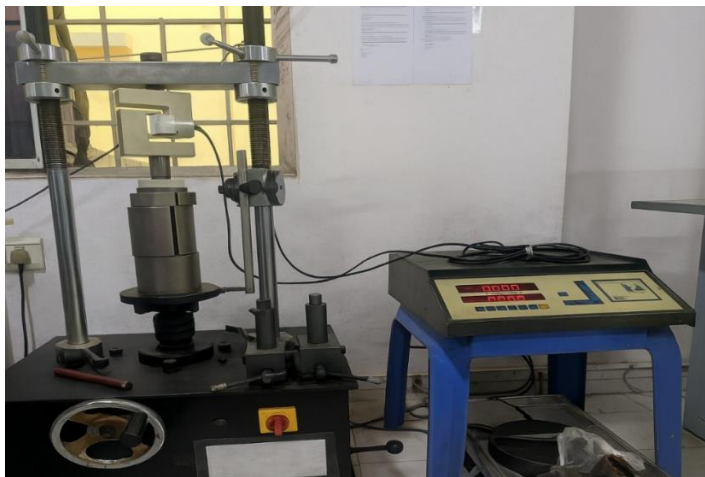
Figure 7. Tensile strength measurement using universal testing equipment.
