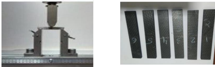
Figure 9. ILSS testing and specimens.
