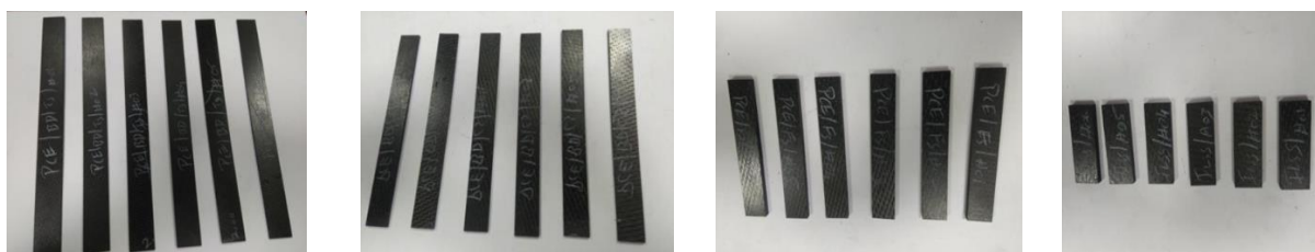
Figure 5. Tensile, compression, flexural, ILSS test specimens.
