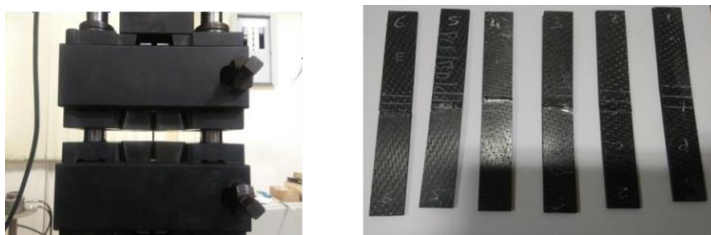
Figure 7. Compression testing & compression tested specimens.
