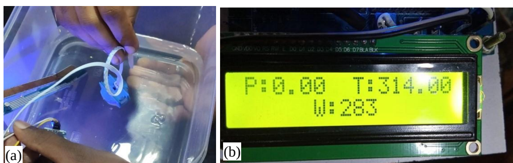
Figure 8. (a)Turbidity Sensor setup, (b) Turbidity Sensor Output display.
