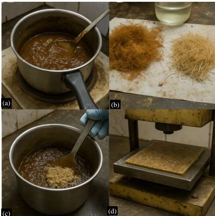
Figure 1. Preparation of TPS–lignin–fiber polymer composites.
