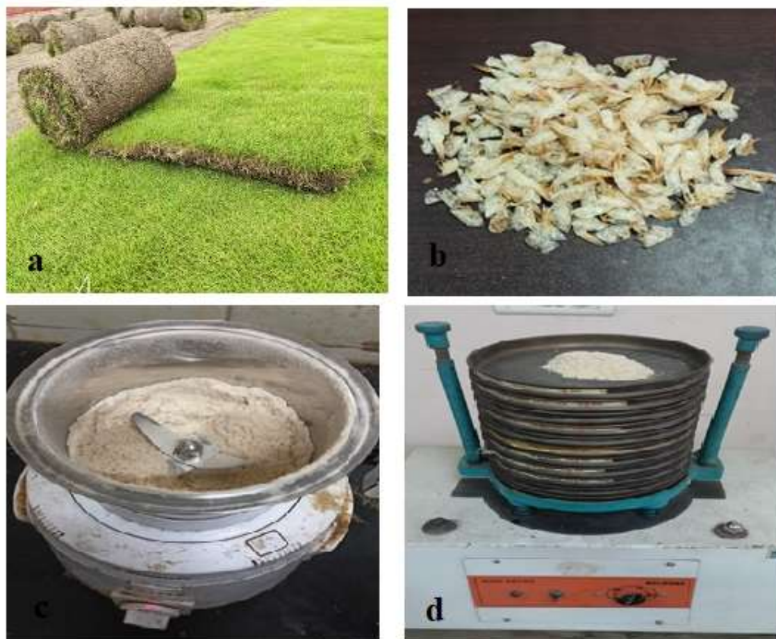
Figure 2. a) Grass Fiber b) Shrimp shell collection c) Blending d) Sieving
