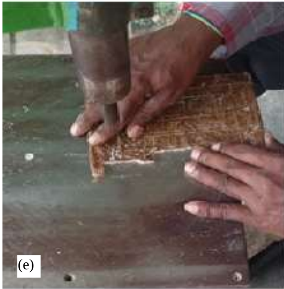
Figure 3. a) Cold Pressing Machine b) Unloading the Cylindrical Sample c) Hand Lay Up Process d) Final FRP Composite e) Cutting according to ASTM models.
