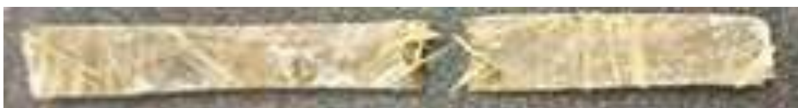
Figure 11. Impact Test Sample After Testing for GFSPRP.
