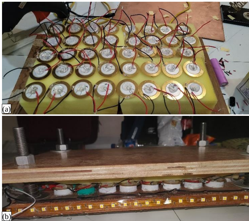
Figure 7. Mechanical stress was provided on transducer pad.
