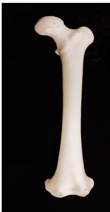
Figure 5. 3D printed femur bone with PLA material using FDM.
