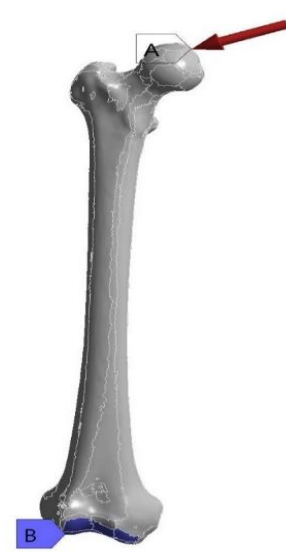
Figure 3. Femur bone with boundary conditions
