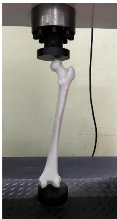
Figure 6. Compression test on 3D-printed PLA femur model.
