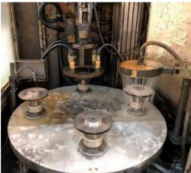
Induction hardening equipment Figure 5. Induction hardening machine.
