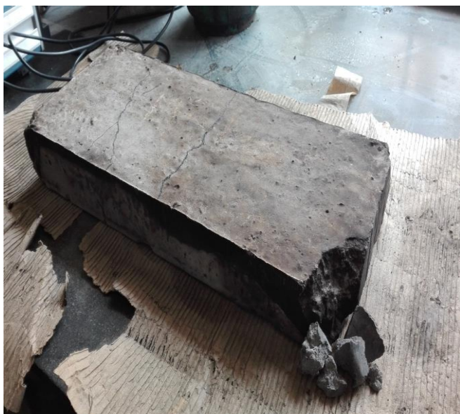
Figure 8. GPC slab P3 – Muffle furnace after 8 hours.
