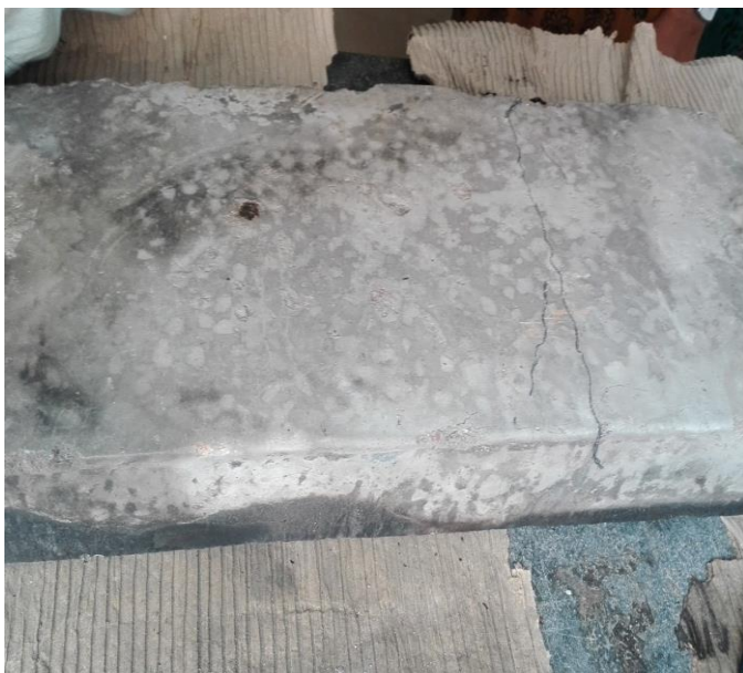
Figure 6. GPC slab P1 – Muffle furnace after 2 hours
