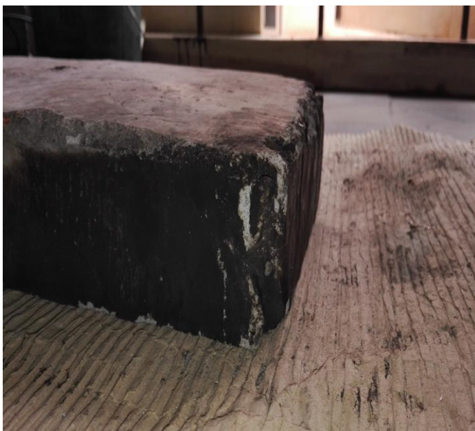
Figure 7. GPC slab P2 – Muffle furnace after 4 hours.
