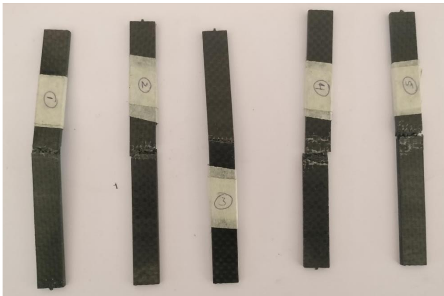
Figure 12. Failed Specimens in Flexural Test
