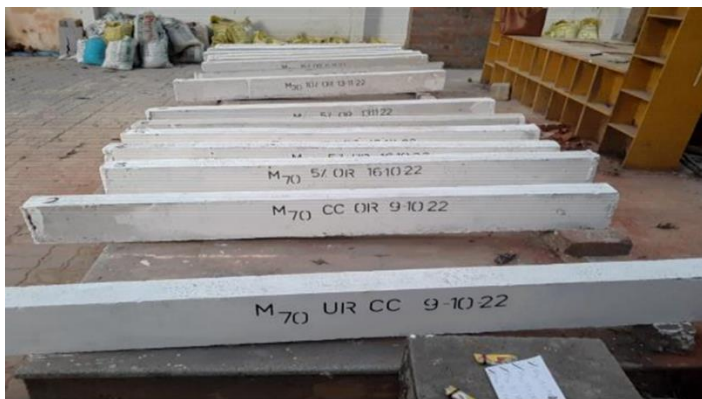
Figure 1. The cast beams are painted white and ready for testing
