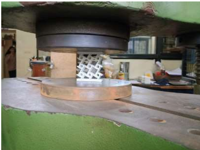
Figure 4. Specimen under compression loading using UTM for compression loading.
