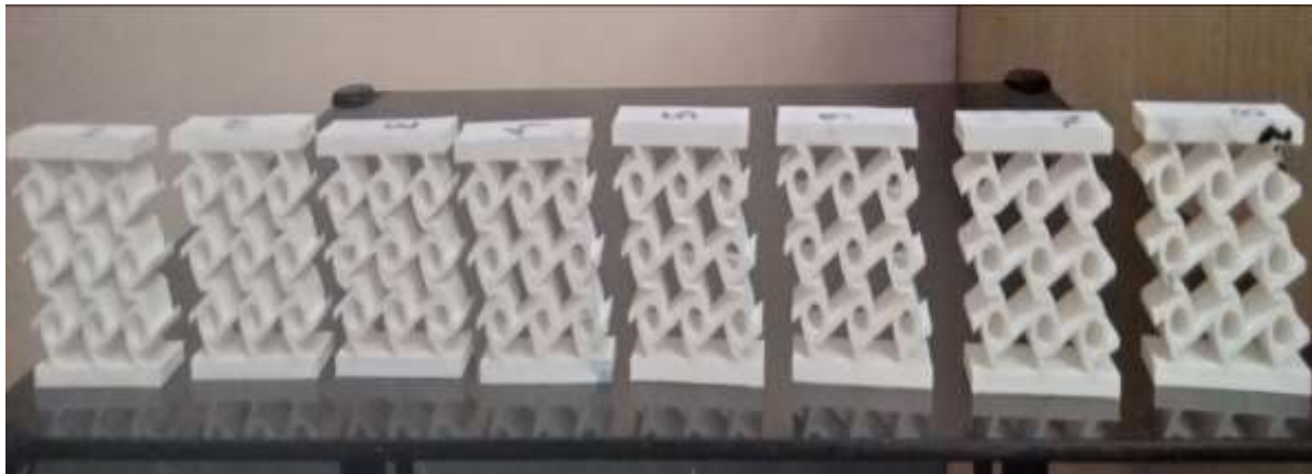
Figure 5. Tetrachiral AUXETIC STRUCTURES after compression testing.
