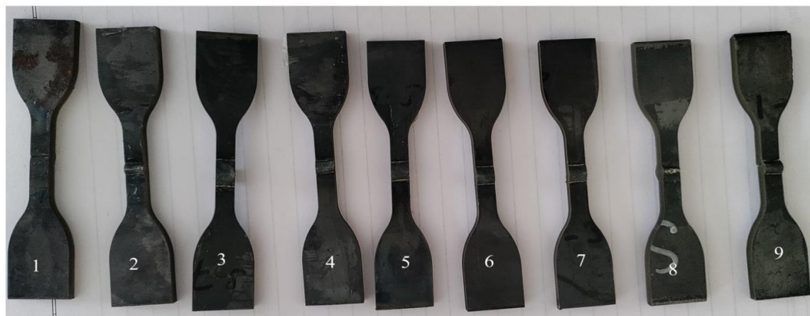
Figure 3. Robotic pulse MIG welding Specimens for tensile test
