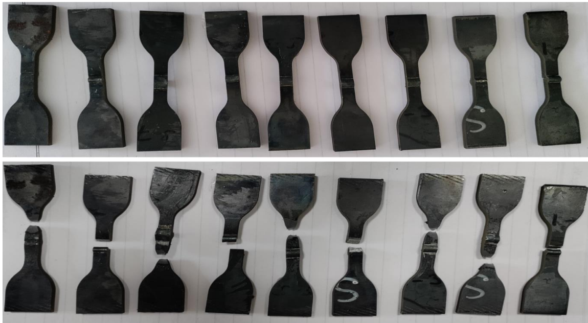
Figure 7. Fracture samples of tensile test
