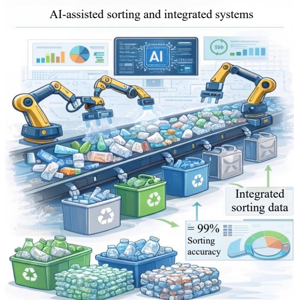
Figure 5. Schematic representation of AI-assisted sorting integrated within advanced recycling systems. In this, artificial intelligence-based systems employing computer vision, near-infrared (NIR) spectroscopy, and robotic separation enhance feedstock purity by identifying and segregating plastics according to polymer type, and color.
