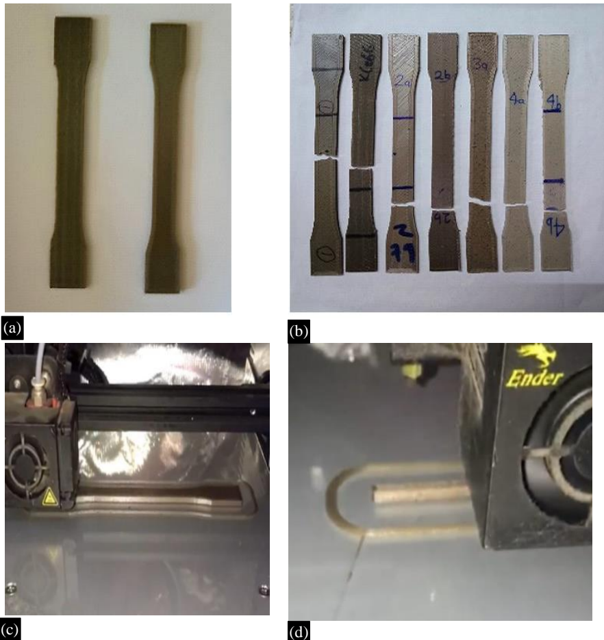
Figure 3. Tensile test specimens as per ASTM D638 a) and b) Tensile specimens as per ASTM D638; c) flat to bed and d) on edge orientation.
