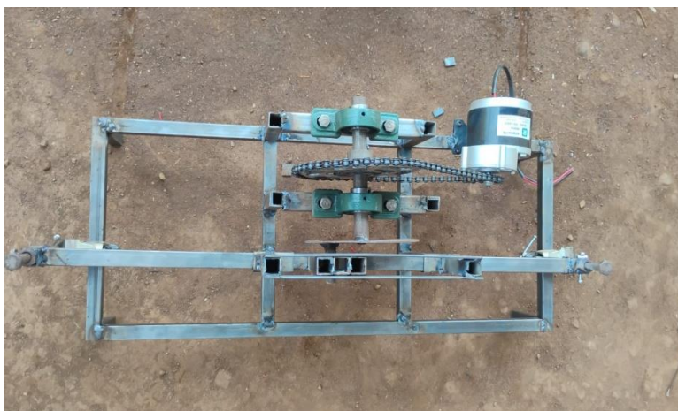
Figure 3. Motorised dual side shaping machine with IoT integration
