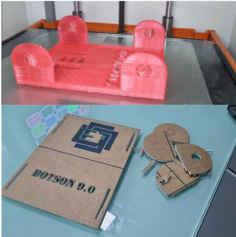
Figure 3. Images of the 3D Printing and Laser Cutting Processes Used in the Fabrication of the Chassis.
