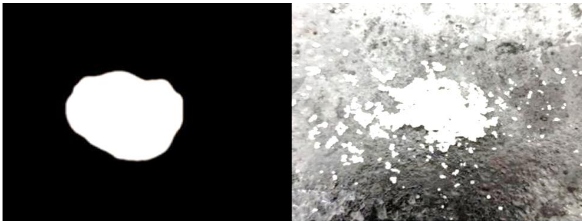
Figure 2. The image shows a light-cured nanoparticle composite block and its powdered form
