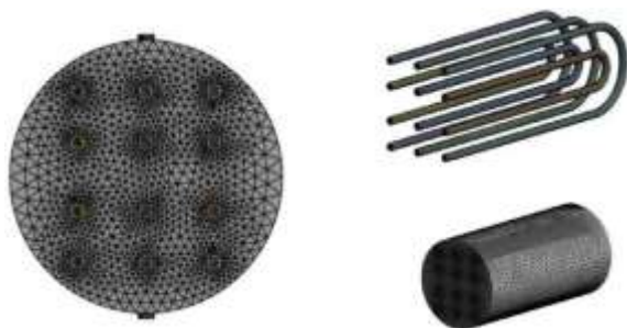
Figure 4. Mesh details with tetrahedral meshing.
