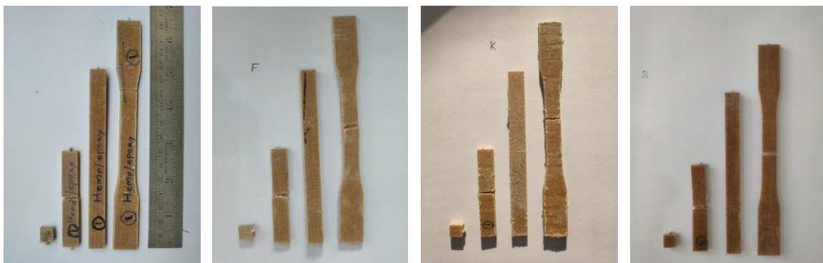
Figure 4. Test specimen after test: (a) Hemp/epoxy, (b) Flax fiber/epoxy, (c) Kenaf/epoxy, and (d) bamboo/epoxy.
