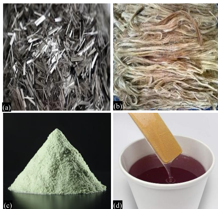
Figure 1. The following materials: (a) Basalt fibre; (b) Kenaf fibre; (c) Titanium dioxide and (d) Resin for binding.
